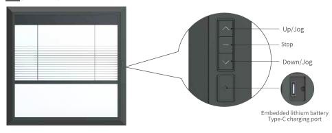
Instructions: (Take A13 button transmitter as an example, for other transmitters, please refer to the corresponding transmitter manual.) Pairing transmitter and motor: Repeating the pairing steps to delete current pairing. A motor can store up to 5 channels, add new channel, the
